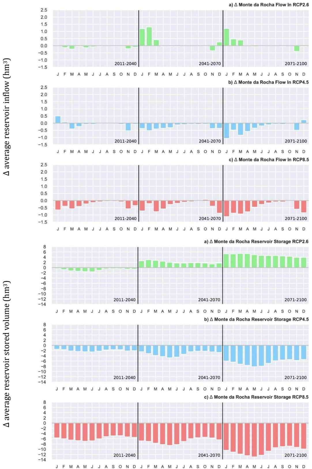
Figure 13 - Projected changes (multi-model ensemble mean) in averaged inflow (top) and volume stored (bottom) in  $\text{hm}^3$  for the Monte da Rocha reservoir, located in River Basin District RH6. Three future periods are shown: 2011-2040, 2041-2070, and 2071-2100, under all emission scenarios – RCP2.6 (green), RCP4.5 (blue) and RCP8.5 (red).
