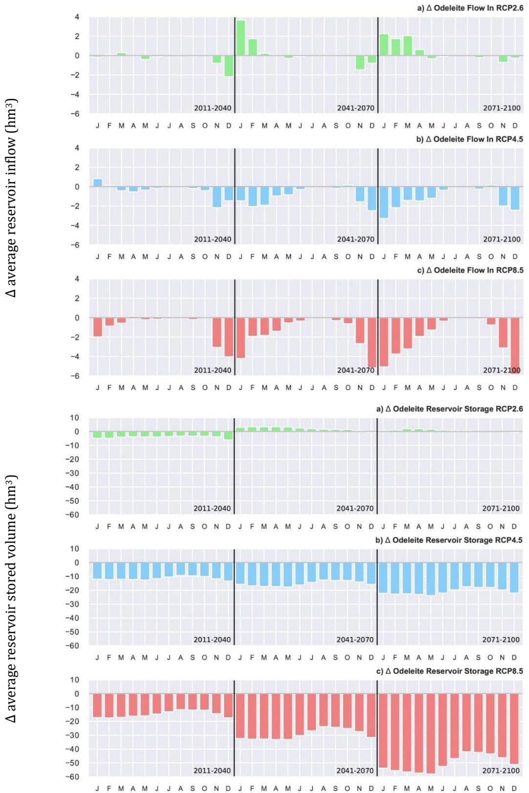
Figure 18 – Projected changes (multi-model ensemble mean) in averaged inflow (top) and volume stored (bottom) in  $\text{hm}^3$  for the Odeleite reservoir, located in River Basin District RH8. Three future periods are shown: 2011-2040, 2041-2070, and 2071-2100, under all emission scenarios – RCP2.6 (green), RCP4.5 (blue) and RCP8.5 (red).
