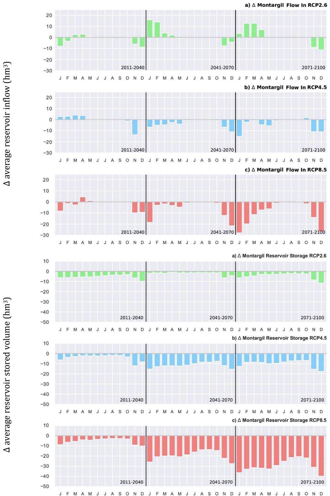
Figure 12 – Projected changes (multi-model ensemble mean) in averaged inflow (top) and volume stored (bottom) in  $\text{hm}^3$  for the Montargil reservoir, located in River Basin District RH5. Three future periods are shown: 2011-2040, 2041-2070, and 2071-2100, under all emission scenarios – RCP2.6 (green), RCP4.5 (blue) and RCP8.5 (red).
