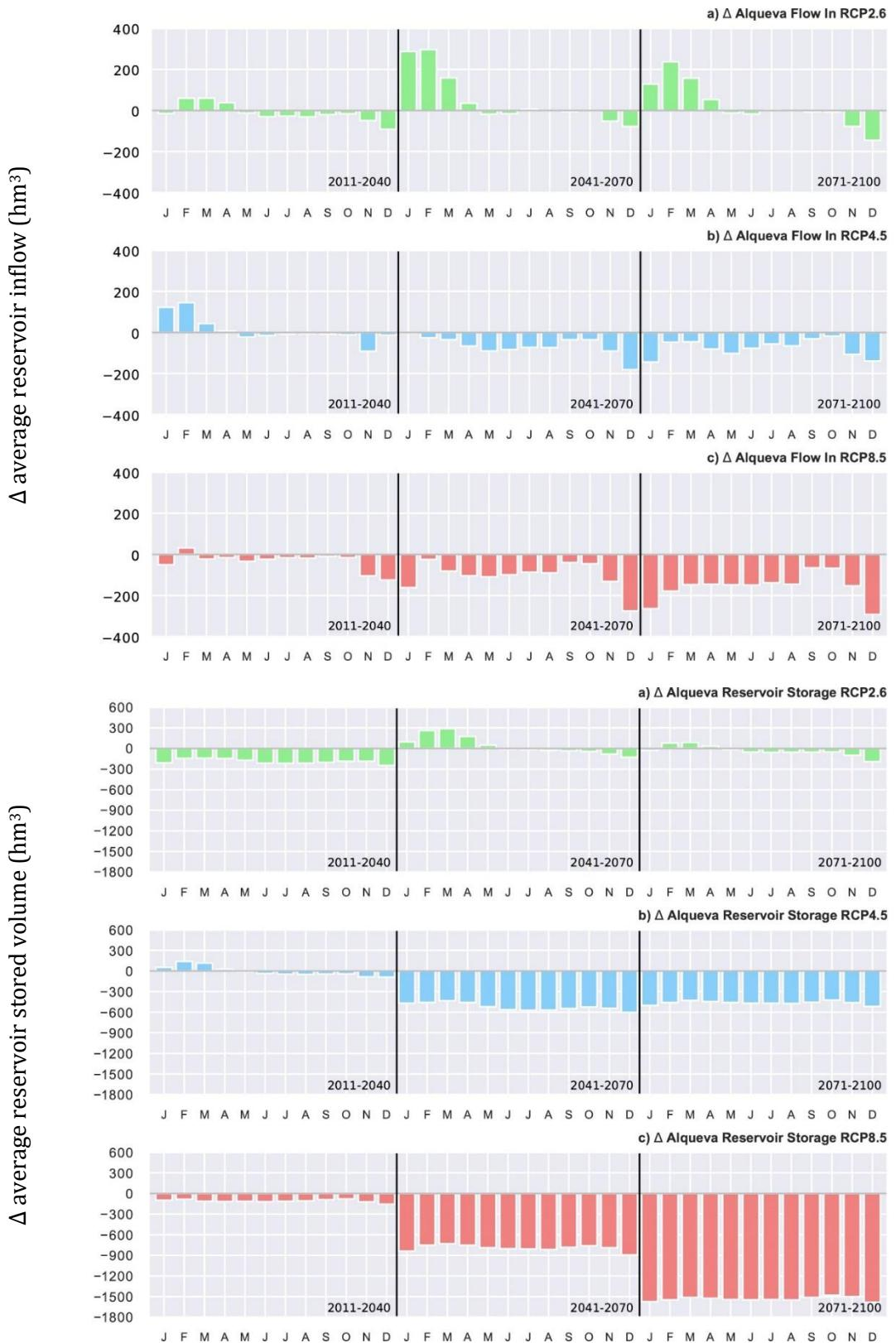
Figure 15 – Projected changes (multi-model ensemble mean) in averaged inflow (top) and volume stored (bottom) in  $\text{hm}^3$  for the Alqueva reservoir, located in River Basin District RH7. Three future periods are shown: 2011-2040, 2041-2070, and 2071-2100, under all emission scenarios – RCP2.6 (green), RCP4.5 (blue) and RCP8.5 (red).
