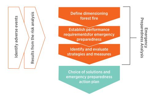
FIGURE 4. Simplified figure based on NORSOK Standard Z-13 showing the relationship between risk and emergency preparedness analyses and the three steps in the emergency preparedness analysis.
